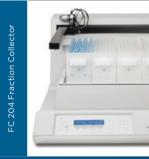
The FC 204 Fraction Collector is a large-bed fraction collector capable of handling test tubes, vials, and up to eight shallow or deep well microplates. Fractions can be collected by drop, peak, or time, and the collector can be used with any HPLC system.
